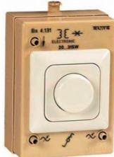
BS 4.131 Dimmer for Electronic Transformers For the connection of electronic transformers, with a rotary knob for continuous brightness adjustment and an integrated pressure change-over switch. For use with electronic transformers and lamps (resistive loads), 20 ... 315 W. Ripple free and short circuit proof with overload protection and Softstart. Operating voltage: 230 V AC.
