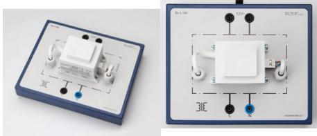
BS 4.190 Transformer Primary: 230 V AC, 50 ... 60 Hz, connection via 4 mm safety sockets Secondary: 11.6 V AC, 50 VA connection via 2 mm safety sockets
