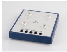
**BS 4.154 Sockets for LV-Halogen Lamps** Experimental module with 4 sockets for low-voltage halogen lamps.
