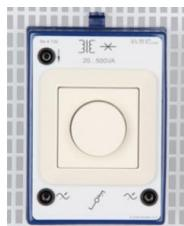
BS 4.130 Dimmer for Inductive / Resistive load Dimmer for Inductive / Resistive load With rotary button for continuous brightness adjustment and an integrated pressure change-over switch. For the connection of dimmers, transformers 20 ... 500 VA and lamps 20 ... 500 Watts (phase control). Interference-proof according to VDE 0639. Operating voltage: 230 V AC.
