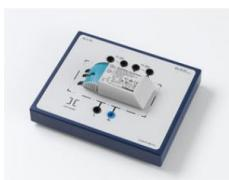
BS 4.191 Electronic Transformer Primary: 230 V AC, 50 ... 60 Hz connection via 2 x 4 mm safety sockets Secondary: 11.8 V, 35 ... 105 W connection via 2 x 2 mm safety sockets.
