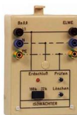
BS 0.8 Ground-leakage monitor The fault to ground is indicated by a signal lamp. After elimination of the fault to ground, the normal function may be re-established by operation of the pushbutton "Reset". The pushbutton "Test" is used for verifying the function of the equipment. The sensitivity may be selected with a switch.
