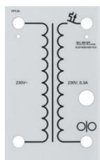
Mask VP 0.9c Isolating Transformer
