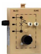
BS 0.3 Current-consuming equipment - "Filament lamp" The module is supplied by way of the service cable with grounding-type plug. The sockets located in parallel to the lamp symbol are used for the production of short-circuits to exposed conductive parts.
