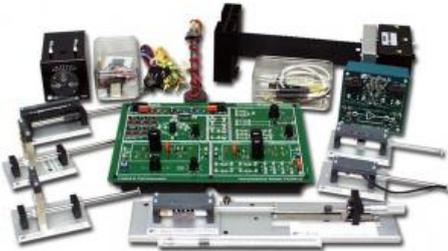
The measurements package is an instrumentation module with signal conditioning circuitry and includes a wheatstone bridge, oscillator, operational amplifier, discriminator and power amplifier.
